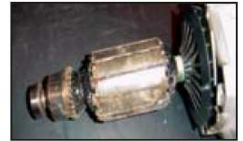
Armature burnt out (overloaded)
