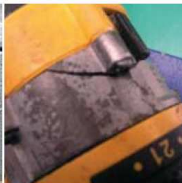
Cracks on dropped unit
